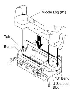
Figure 21 - Installing Middle Log (#1)
